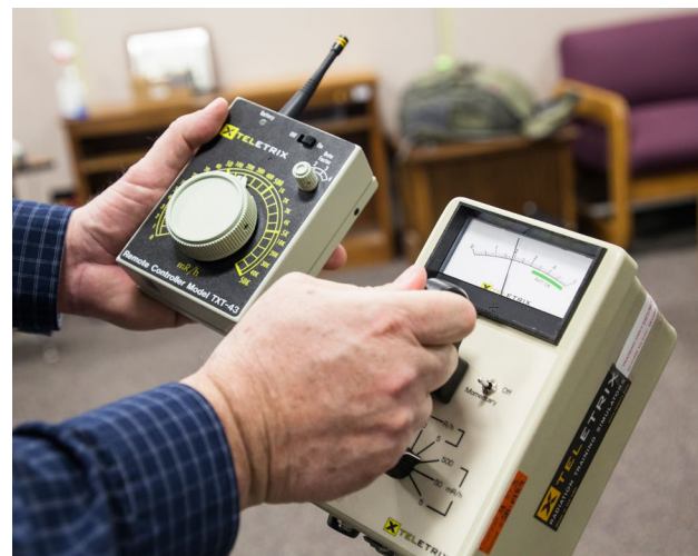
Radiation instrumentation used for training can be remotely controlled by the instructor.
